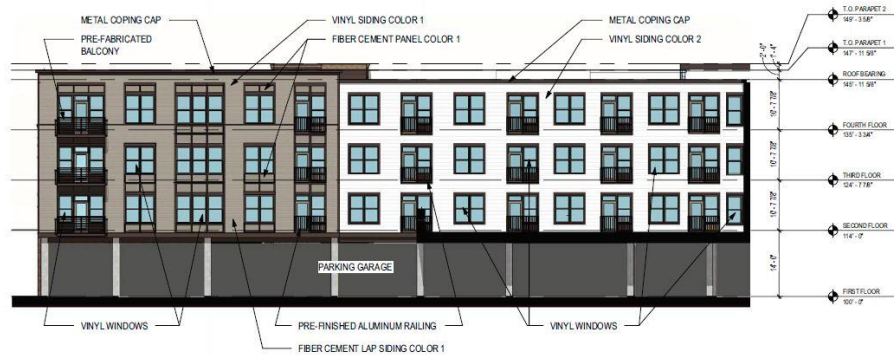
west elevation - amenity deck 1/16" = 1'-0"
