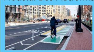
Modular rubber bus platforms for safer transit operations and potential for protected bike lanes
