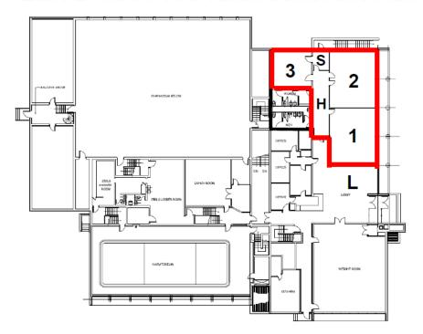
Renovation Area: Rooms 1, 2, 3; the hallway (H) and the storage closet (S) at the end of the hallway. The wall between Rooms 1 & 2 will be removed and the wall facing the lobby (L) will be opened to create a main entrance to the center.
